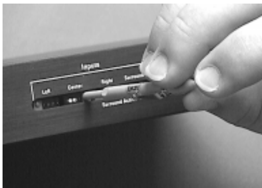
Figure 4-1 Adjusting the Center Input Trim Control
