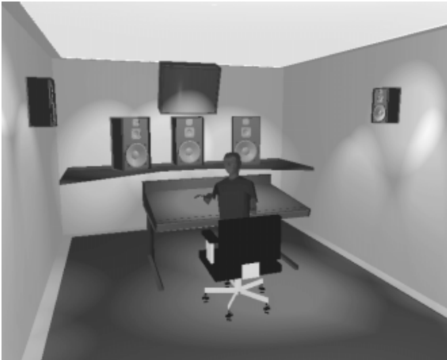
Figure 2-16 Vertical Location of Surround Speakers in Control Room
