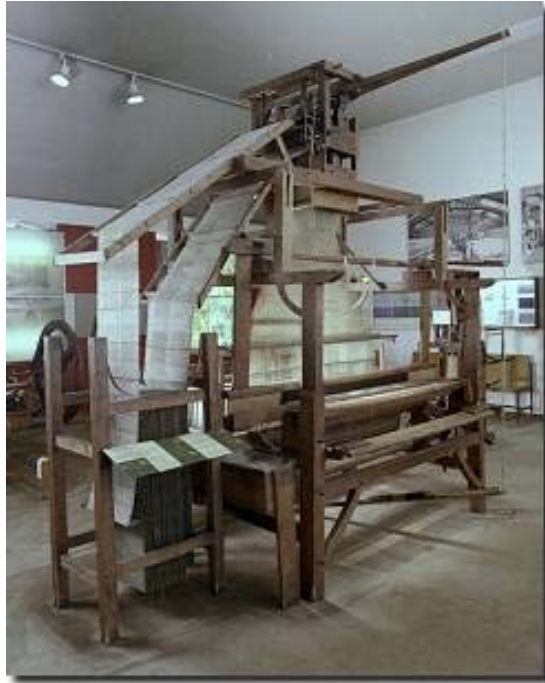
Figure 6.2 An image of the Jaquard loom. Note the punch card apparatus to the left of the device. Jacquard was able to mechanise iterations of patterns in the final fabric through looping the punch cards. Courtesy of Deutsches Museum 2001.
