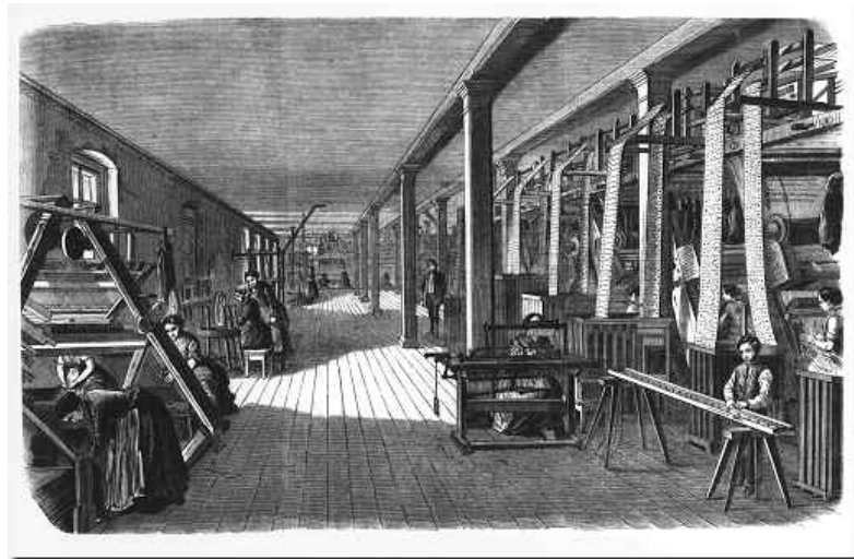
Figure 6.3 Jacquard pattern looms in the factory Gevers & Schmidt in Schmiedeberg (Silesia, Germany). The pattern is entered via the punched cards. The image is a wood engraving from 1858. Note the depiction of women working on the looms. Courtesy of Deutsches Museum 2001.
