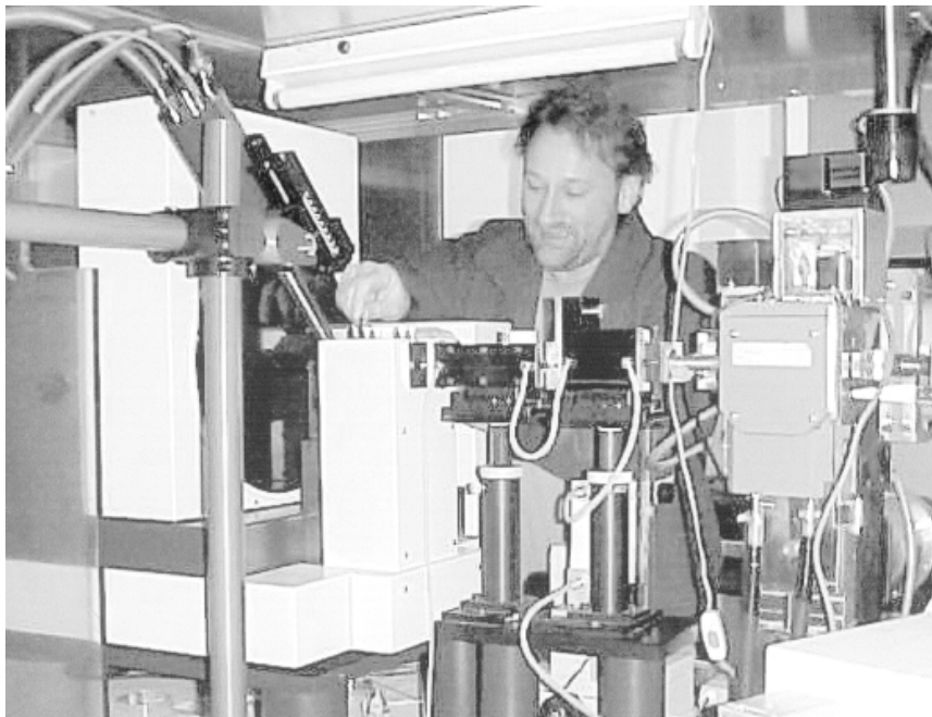
Dr Matthew Wilce mounting a crystal in preparation for an X-ray diffraction experiment.
