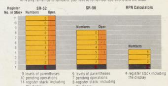
A calculator with full AOS remembers both the numbers and functions in its register stack. And performs them according to algebraic hierarchy. As more operations become pending, the stack fills up (see diagram). Finally, when the equals key is pressed, the operations in the register stack are performed to give you the correct answer (15.21311475). Automatically.
