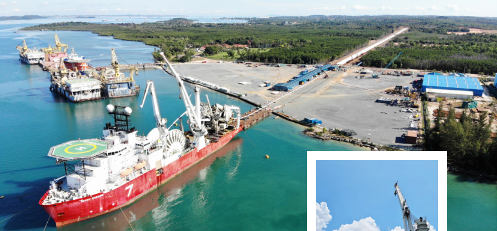
Above: The Seven Oceans pipelay vessel being loaded in Bintan, Indonesia, with pipe destined for the Julimar project off the north west of Western Australia; right, it is believed the 18 inch diameter corrosion-resistant alloy pipe is the biggest diameter ever reeled.
