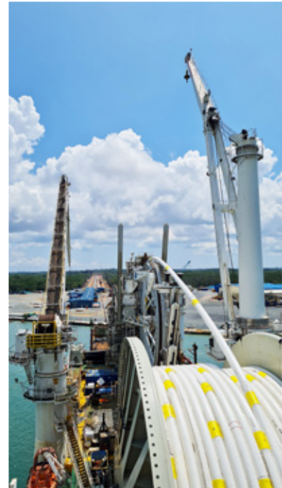
Above: The Seven Oceans pipelay vessel being loaded in Bintan, Indonesia, with pipe destined for the Julimar project off the north west of Western Australia; right, it is believed the 18 inch diameter corrosion-resistant alloy pipe is the biggest diameter ever reeled.
