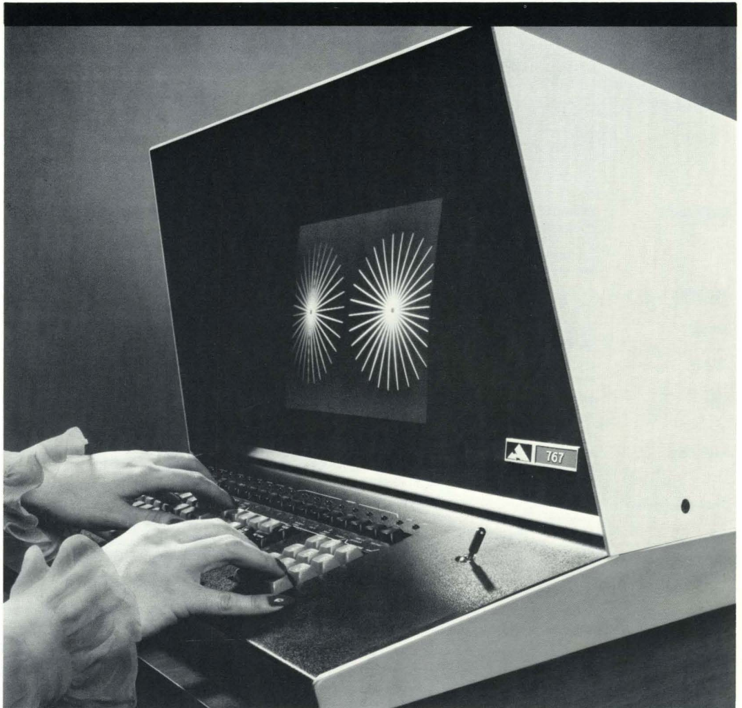
The AED767 graphics terminal is sufficiently compact to fit easily on a desktop. It comes complete with keyboard, joystick, I/O ports, and all electronics. Optional display monitors are available from AED.
