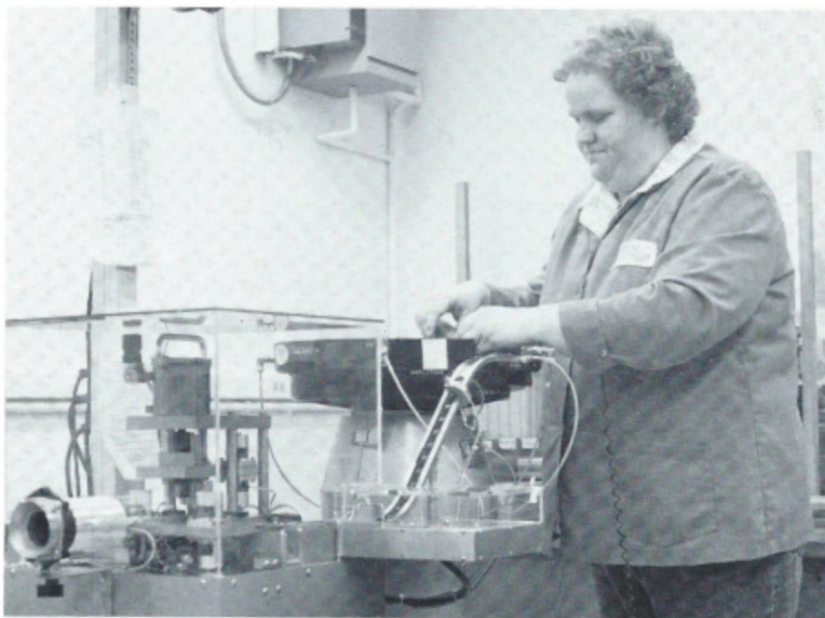
Shirley Thumberry loads raw chips into the RISI machine for preparation before assembly into a circuit board. The RISI machine prepares 1,000 chips an hour.
