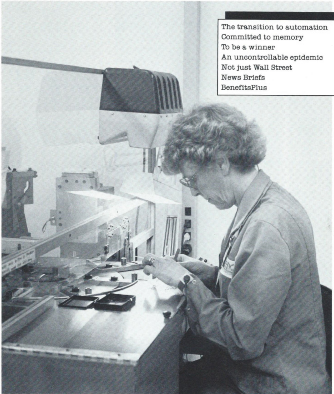
People at Cray Research's Rice Lake facility have installed automated equipment to help save time and increase quality. Above, Judy Johnson feeds resistors into an automated preparation machine.
