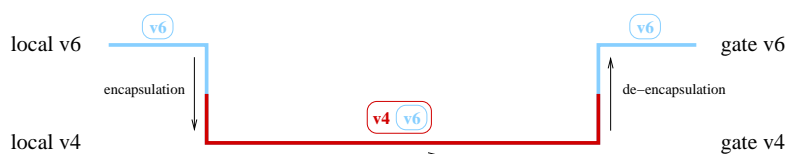
Figure 23-2. A frequently used method for transition is tunneling IPv6 in IPv4 packets
